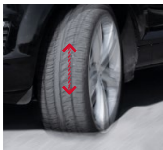
STATIC IMBALANCE: The wheel has a tendency to jump.
