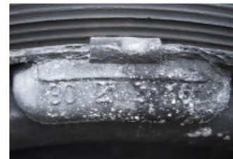
UNCOATED WEIGHTS: Contact corrosion of surface.
