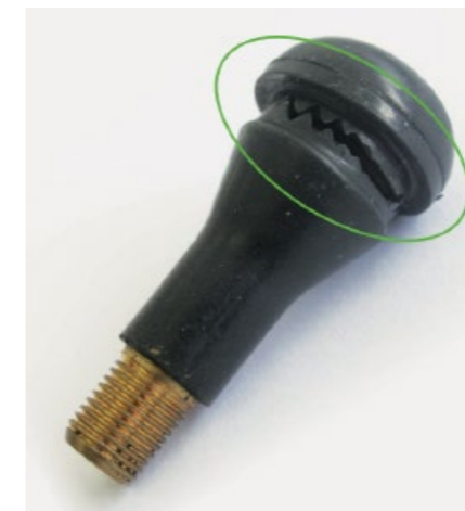
Old, torn valve
