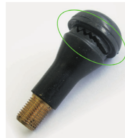
Old, torn valve
