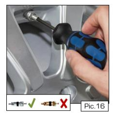
Finally, screw the new nickel plated valve core in the valve (see Pic. 16). Ensure the right torque. Now you can go on with the usual steps of a wheel assembly.
