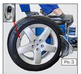
It is important that the TPMS Sensor is on the opposite side of the bead breaker, when the tyre is pressed down on the rim (see Pic.3).
