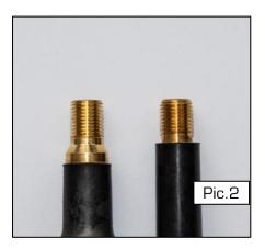
Also in case of a snap-in valve, there exist some characteristics which give hints that a direct TPMS is installed. The rubber coating ends in the most cases 6mm before the thread. The end of the rubber coating for standard snap-in valves without sensor is directly on the thread (see Pic.2).
