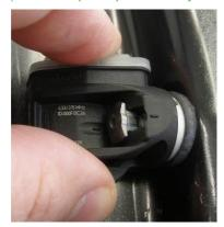
If all the adjustable angle space is not used, it may cause the grommet not to lie correctly on the rim which can lead to leaks.
