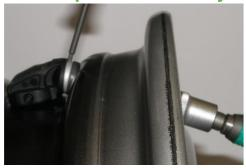
The cross-bore in the base of the valve is for disassembly. The disassembly pin can be used to loosen a stuck hexagonal nut.
