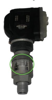
The shear-collar breaks at less than 3.5 Nm
