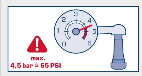
Rubber Valves can be used up to a pressure of 4,5 bar.
