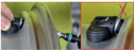
After assembly, check that the housing is seated firmly!
