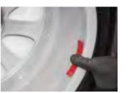
Attach the weight centrally on the calculated position, making sure that the weight is parallel to the edge of the rim.
