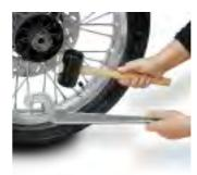
are attached to the spoke nipple, using HOFMANN POWER WEIGHT impact tool no. 385/1. This is the only way to avoid installation errors, as the HOFMANN POWER WEIGHT tool transfers the force necessary for ensuring that the weight is clamped securely and precisely. An assembly with other tools or the use of weights, which are compressed only with pliers, can cause the weights to detach during driving.
