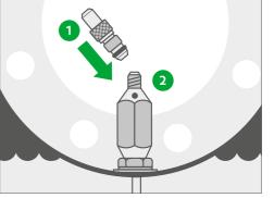
■ Screw valve core housing 1 into water filling valve 1.
